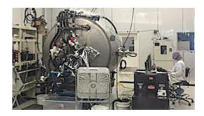
beyond Earth. The 100K cleanroom also features a thermal vacuum test chamber in which instruments and spacecraft can be tested under the temperature and vacuum conditions they will experience in space. Watch this video
