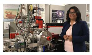
extraterrestrial samples, the primary advantage of the NanoSIMS over other analytical tools is its ability to deliver high spatial resolution even on areas smaller than 1 micron. Watch this video for a behind the scenes look inside the NanoSIMS lab.
